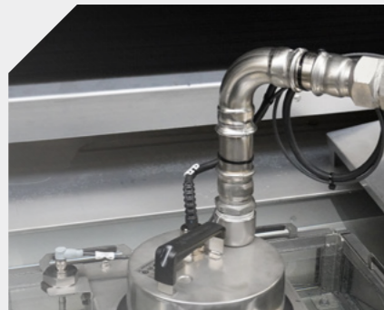
immersion pump/潜水泵
